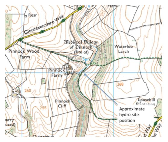
Small scale, run-of-river hydro technology is well established. Turbine choice is largely driven by head, where there is disagreement about the exact definitions of low and high head, but the Pinnock Farm hydro, at around 5m head, would be classified as low head. Various turbine options exist for low head sites such as this.
